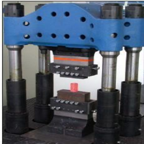
Fig.1 Open-die Hot Forging Operation
