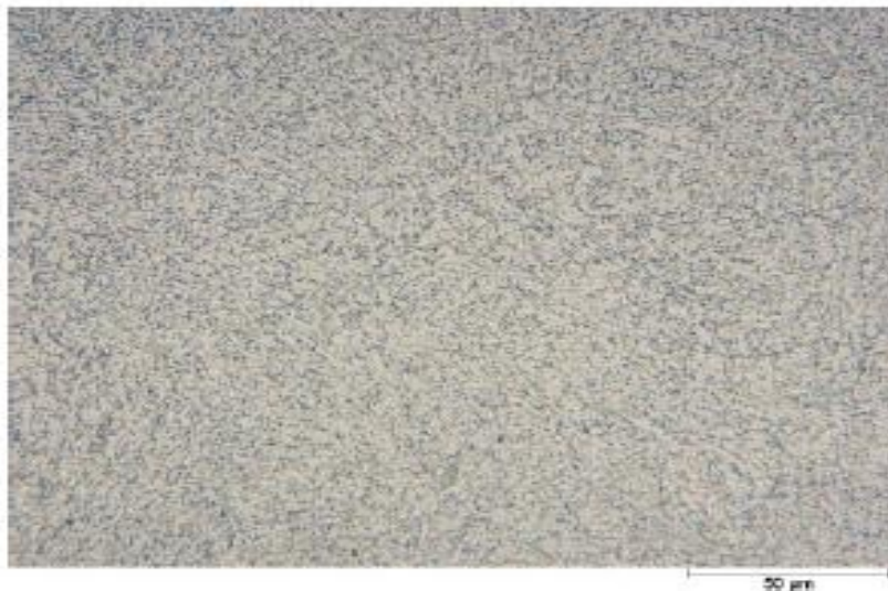
(AISI H13), as annealed structure Microstructure, Etched with 2% nital
