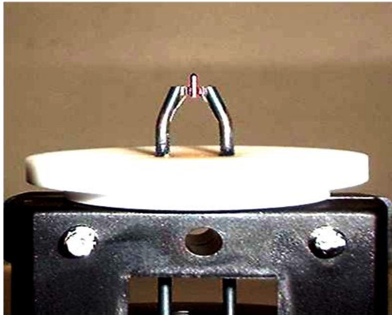
Fig ;4 Conventional tungsten hairpin filament electron gun
