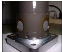
Beryllium windows on the X-ray tube, one for each port.
