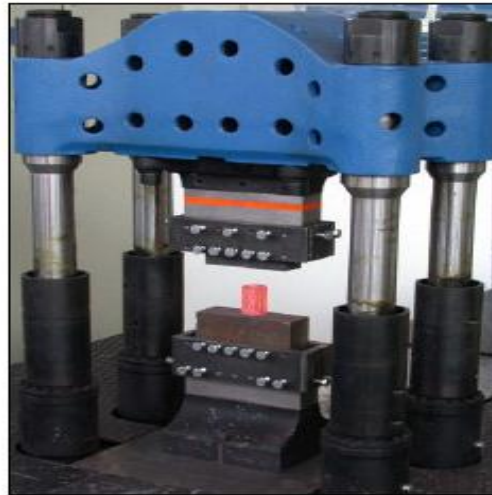
Fig.1 Open-die Hot Forging Operation
